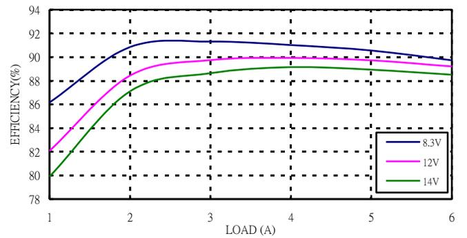
**Figure 6:** Converter efficiency vs. output current (3.3V output voltage)
