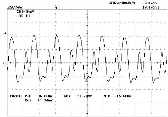
Figure 9: Output ripple & noise at 12Vin, 5.0V/6A out
