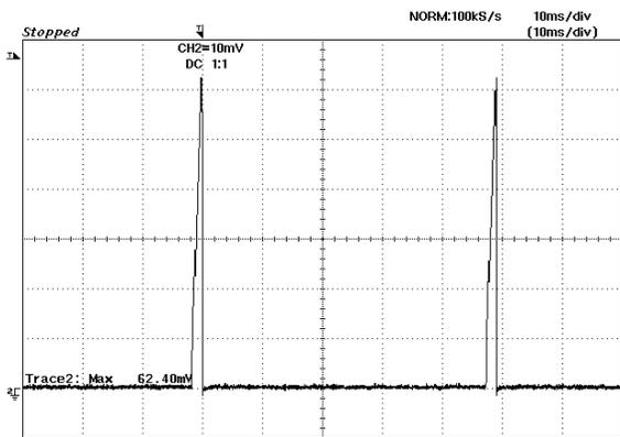
**Figure 15:** Output short circuit current 12Vin, 0.75Vout (5A/div)
