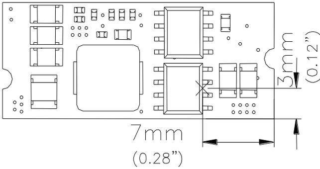
**Figure 31:** Temperature measurement location
