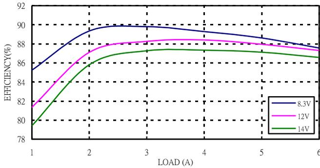
**Figure 5:** Converter efficiency vs. output current (2.5V output voltage)
