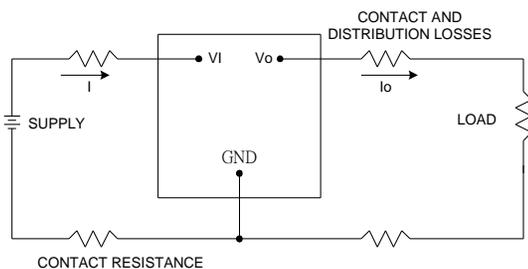
**Figure 19:** Output voltage and efficiency measurement test setup
