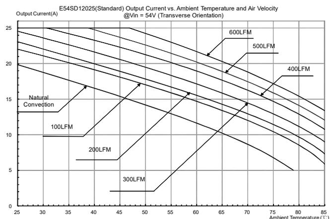
Figure 23: Output current vs. ambient temperature and air velocity @Vin=54V(Transverse Orientation, airflow from Vin- to Vin+, without heat spreader)
