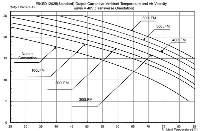
Figure 22: Output current vs. ambient temperature and air velocity @Vin=48V(Transverse Orientation, airflow from Vin- to Vin+, without heat spreader)
