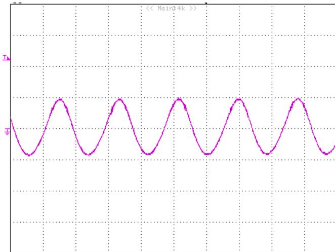
**Figure 14:** Output voltage ripple at nominal input voltage and rated load current ( $I_o=25\text{A}$ ) ( $50\text{mV/div}$ ,  $2\mu\text{s/div}$ )
