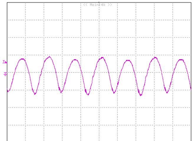
**Figure 11:** Input Terminal Ripple Current,  $i_c$ , at full rated output current and nominal input voltage with  $12\mu H$  source impedance and  $100\mu F$  electrolytic capacitor (0.2A/div, 2us/div).
