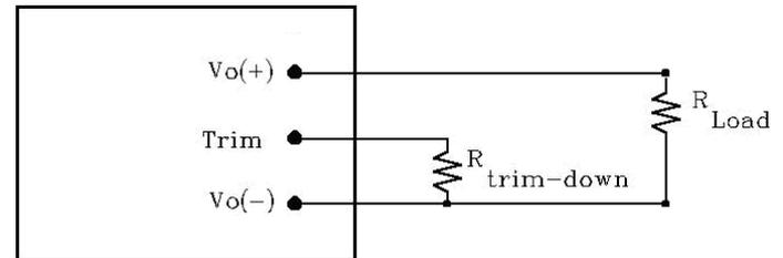
Figure 18: Circuit configuration for trim-down (decrease output voltage)
