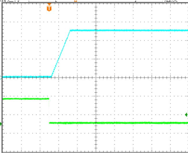
**Figure 5: Remote On/Off (negative logic) at full load**
