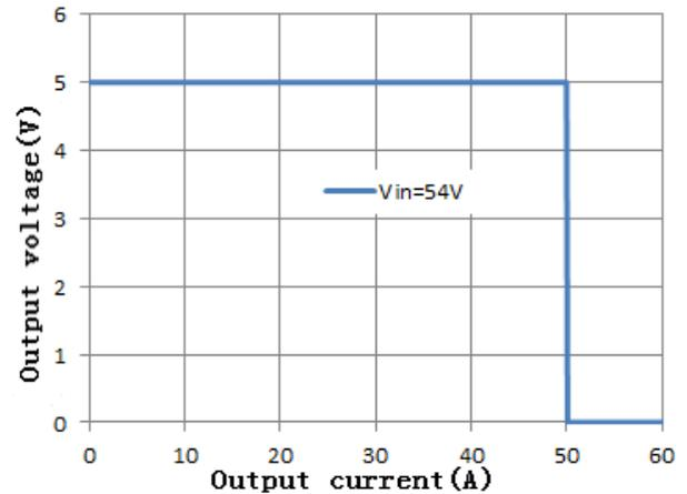
**Figure 4: Output Voltage vs. Output Current showing typical current limit curves and converter shutdown points.**
