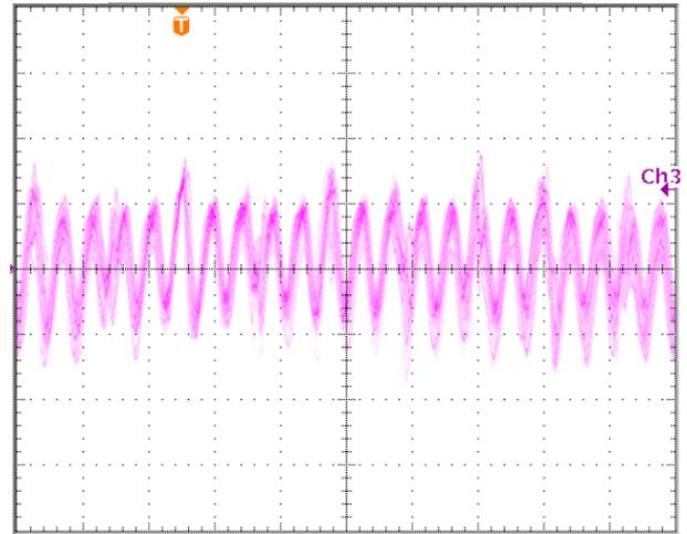
**Figure 10: Input Terminal Ripple Current,  $i_c$** , at max output current and nominal input voltage with  $12\mu\text{H}$  source impedance and  $100\mu\text{F}$  electrolytic capacitor (100 mA/div, 2us/div).
