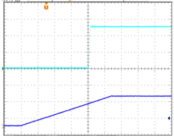
**Figure 6: Input Voltage Start-up at full load**
