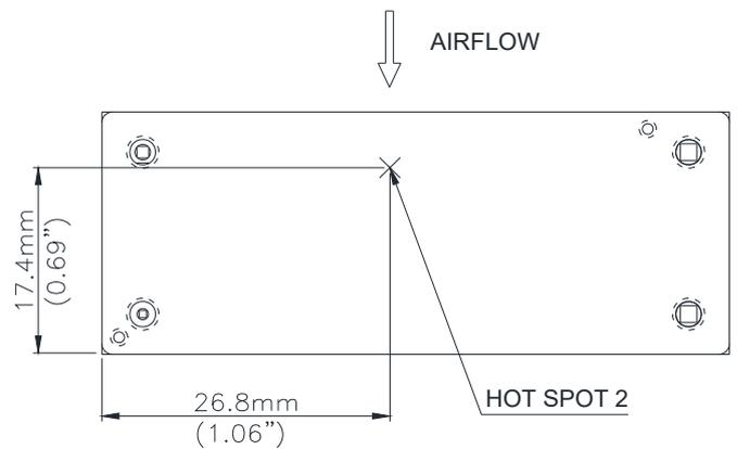
**Figure 19: Hot spot 2 temperature measurement location**
