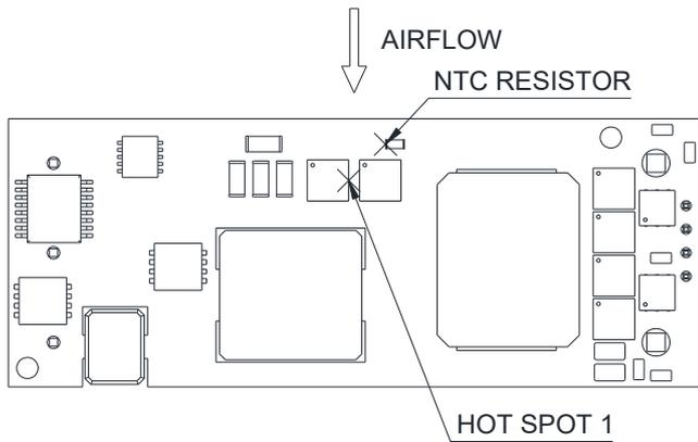
**Figure 17: Hot spot 1 temperature measurement location**
