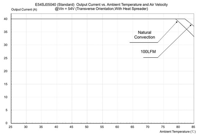
**Figure 20: Output Current vs. Ambient Temperature and Air Velocity @Vin = 54V (Transverse Orientation, Airflow from Vin+ to Vin-, With Base-plate)**
