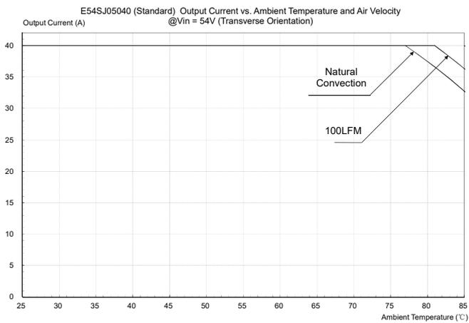
**Figure 18: Output Current vs. Ambient Temperature and Air Velocity @Vin = 54V (Transverse Orientation, Airflow from Vin+ to Vin-, Open Frame)**
