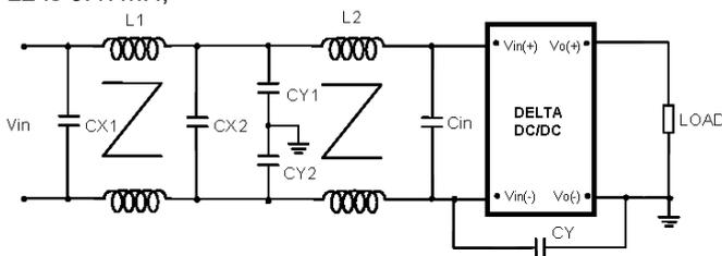
Figure 13-1: Recommended Input Filter
