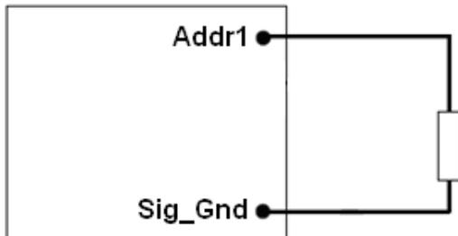
Different PMBUS address is defined by the value of the resistor as below, and +/-1% resistors accuracy can be accepted. If there is any resistance exceeding the requested range, address 127 will be return..
