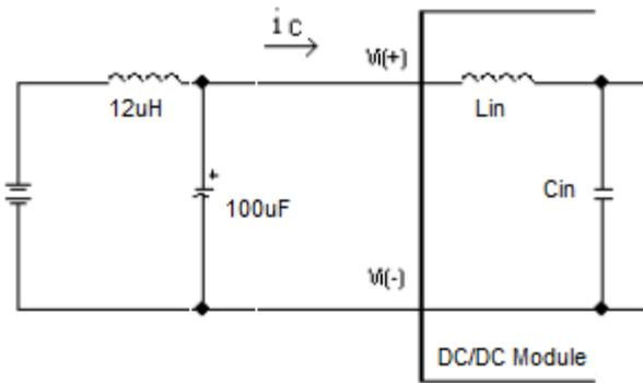
**Figure 9: Test Setup Diagram for Input Ripple Current**
