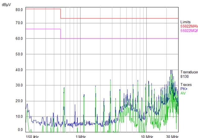
Figure 13-2: Test Result of EMC( $V_{in}=54V$ ,  $I_o=40A$ ).
