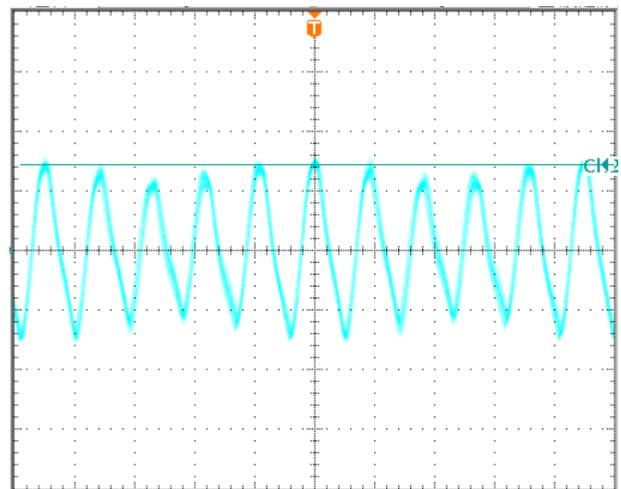
**Figure 12: Output Voltage Ripple and Noise** at nominal input voltage and max load current (20 mV/div, 2us/div)
