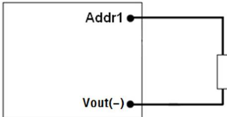
Different PMBUS address is defined by the value of the resistor as below, and +/-1% resistors accuracy can be accepted. If there is any resistance exceeding the requested range, address 126 will be return.
