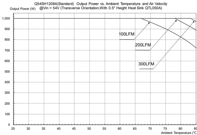
**Figure 20:** Output Power vs. Ambient Temperature and Air Velocity @  $V_{in} = 54V$  (Transverse Orientation, Airflow from  $V_{in+}$  to  $V_{in-}$ , With 0.5" Height Heat Sink QTL050A)
