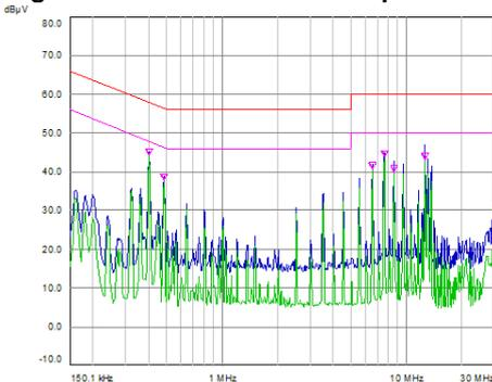
**Figure 13-2: Test Result of EMC ( $V_{in}=54V$ ,  $I_o=84.8A$ ).**
