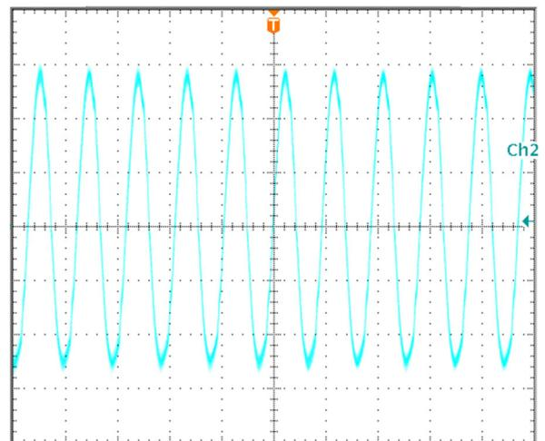
**Figure 12: Output Voltage Ripple and Noise at nominal input voltage and max load current (10 mV/div, 1us/div)**
