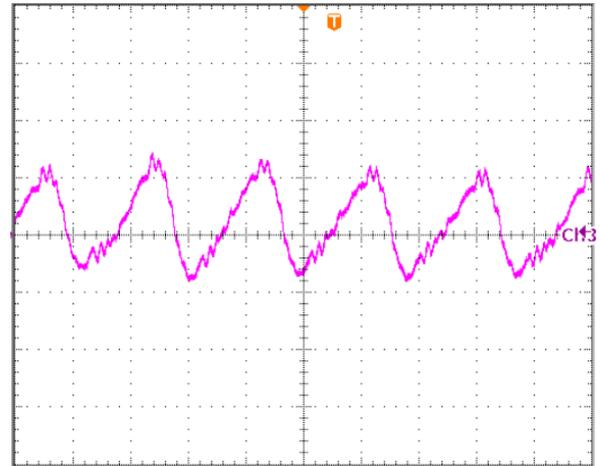
**Figure 10: Input Terminal Ripple Current,  $i_c$ , at max output current and nominal input voltage with  $12\mu\text{H}$  source impedance and  $220\mu\text{F}$  electrolytic capacitor (50 mA/div, 1us/div).**
