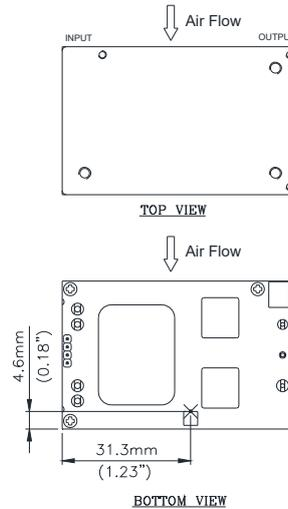
**Figure 17: Hot spot 1 temperature measurement location**
