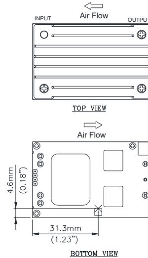
**Figure 21:** Hot spot 3 temperature measurement location
