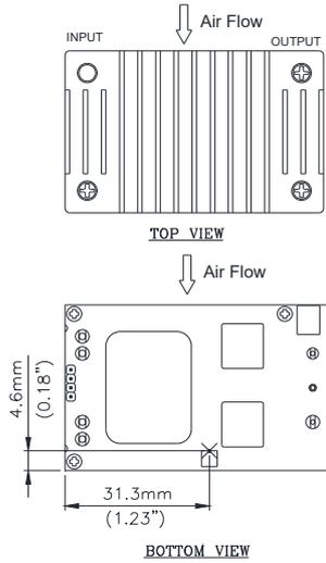
**Figure 19:** Hot spot 2 temperature measurement location
