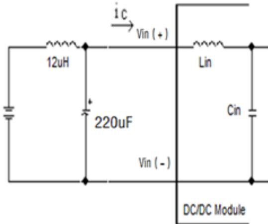
**Figure 9: Test Setup Diagram for Input Ripple Current**
