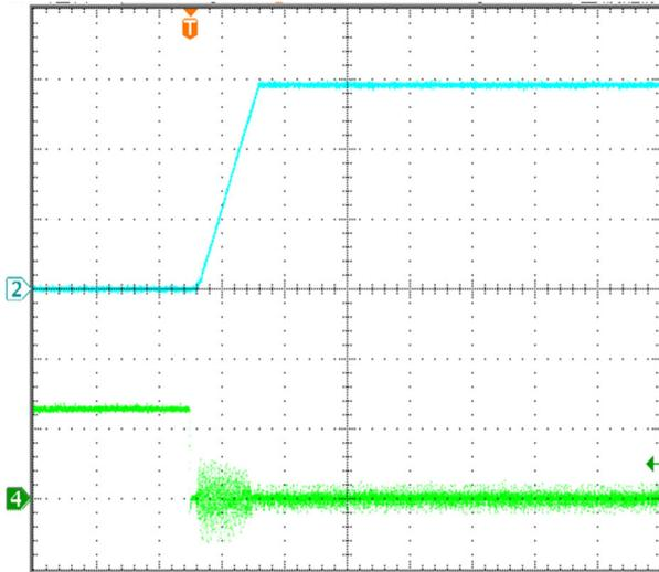
**Figure 5: Remote On/Off (negative logic) at full load**
