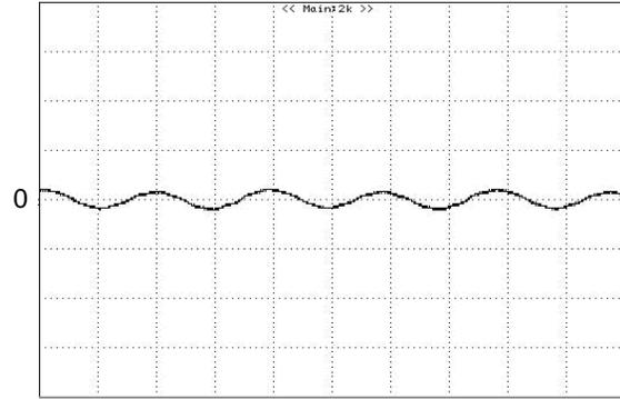
**Figure 10:** Input Terminal Ripple Current,  $i_c$ , at full rated output current and nominal input voltage with 12 $\mu$ H source impedance and 33 $\mu$ F electrolytic capacitor (200 mA/div, 1us/div)
