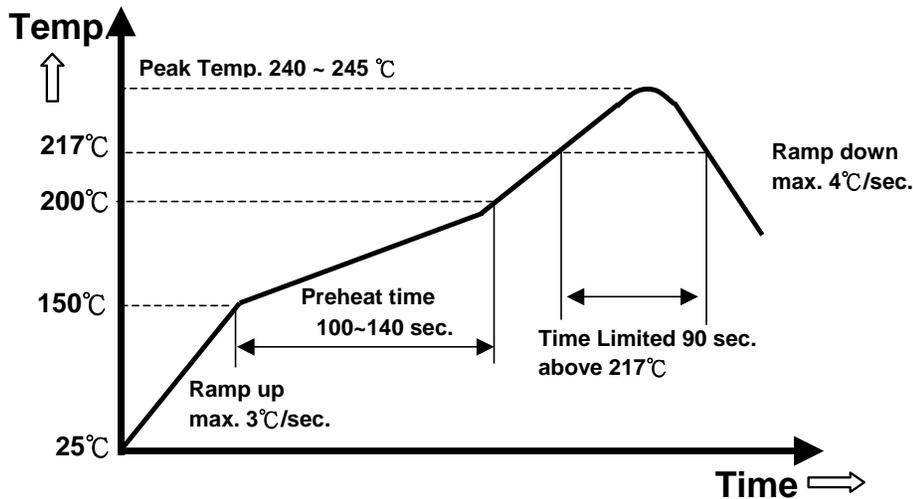
Note: The temperature refers to the pin of V48SH, measured on the pin +Vout joint.
