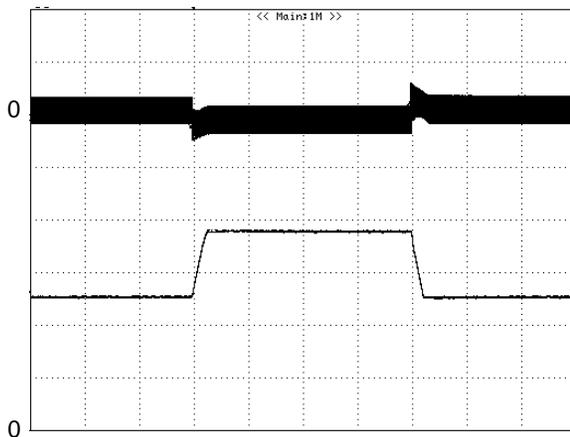
**Figure 8:** Output voltage response to step-change in load current (75%-50%-75% of  $I_{o, max}$ ;  $di/dt = 0.1A/\mu s$ ). Load cap: 10 $\mu F$  tantalum capacitor and 1 $\mu F$  ceramic capacitor. Top Trace:  $V_{out}$  (50mV/div, 500 $\mu s$ /div), Bottom Trace:  $I_{out}$  (10A/div). Scope measurement should be made using a BNC cable (length shorter than 20 inches). Position the load between 51 mm to 76 mm (2 inches to 3 inches) from the module
