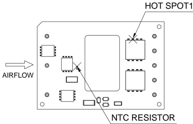
**Figure 19:** \* Hot spot 1 & NTC resistor temperature measured points
