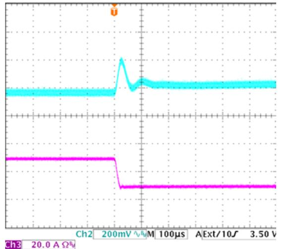
**Figure 9:** Output voltage response to step-change in load current (75%-25% of  $I_o$ , max;  $di/dt = 1A/\mu s$ ;  $V_{in}=48V$ ). Load cap: 1mF tantalum capacitor and 1 $\mu$ F ceramic capacitor. Top Trace:  $V_{out}$  (0.2V/div, 200 $\mu s$ /div), Bottom Trace:  $I_{out}$  (20A/div). Scope measurement should be made using a BNC cable (length shorter than 20 inches). Position the load between 51 mm to 76 mm (2 inches to 3 inches) from the module
