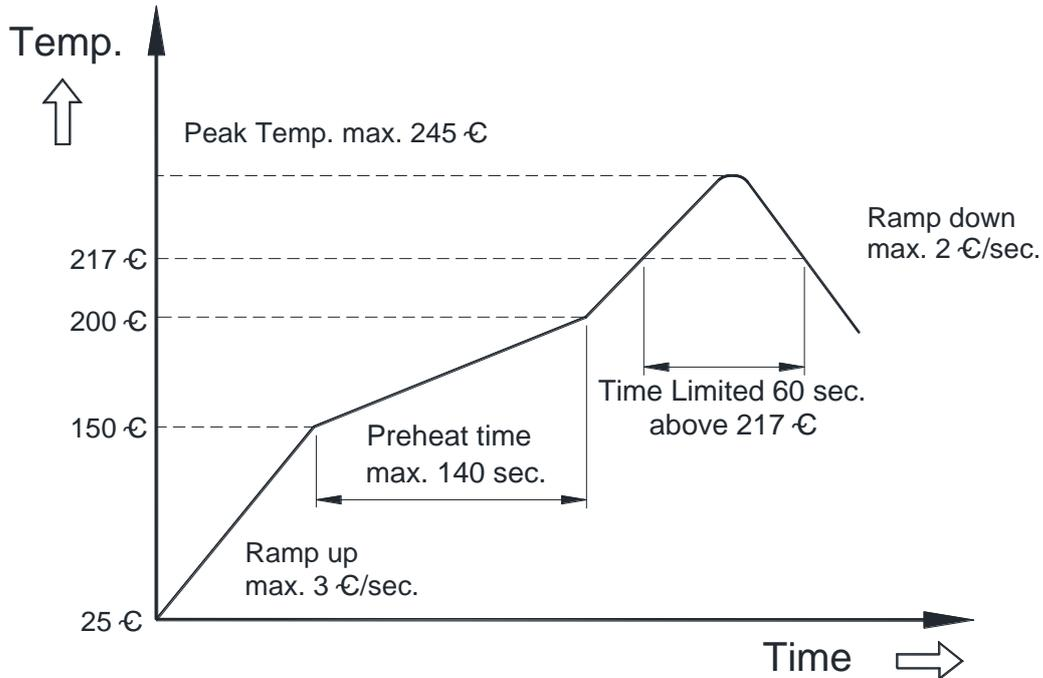
Recommended Temperature Profile for Lead-free Reflow Soldering
