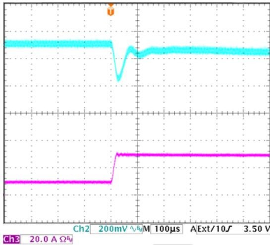
**Figure 8:** Output voltage response to step-change in load current (25%-75% of  $I_o$ , max;  $di/dt = 1A/\mu s$ ;  $V_{in}=48V$ ). Load cap: 1mF tantalum capacitor and 1 $\mu$ F ceramic capacitor. Top Trace:  $V_{out}$  (0.2V/div, 100 $\mu s$ /div), Bottom Trace:  $I_{out}$  (20A/div). Scope measurement should be made using a BNC cable (length shorter than 20 inches). Position the load between 51 mm to 76 mm (2 inches to 3 inches) from the module
