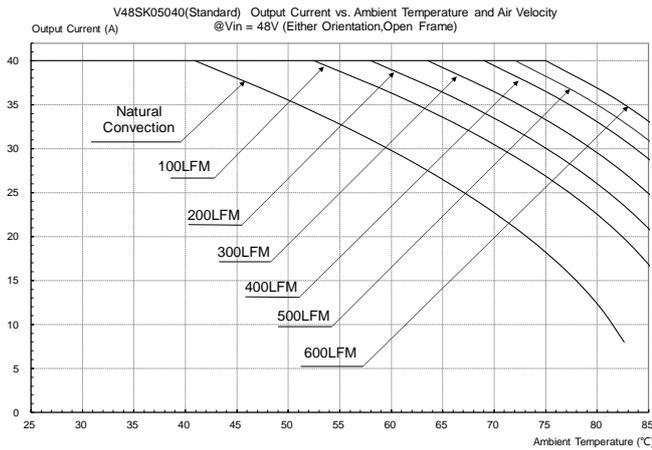
**Figure 19:** Output current vs. ambient temperature and air velocity @Vin=48V(Either orientation, open frame)
