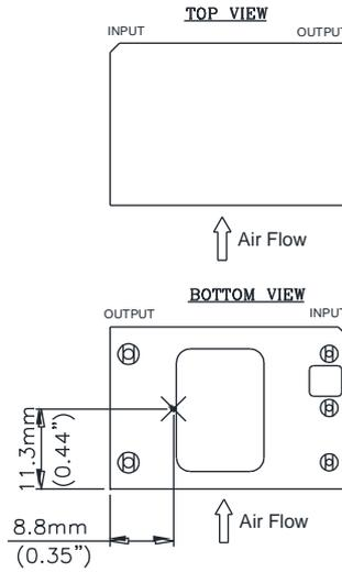
**Figure 20:** \* Hot spot 2's temperature measured point.
