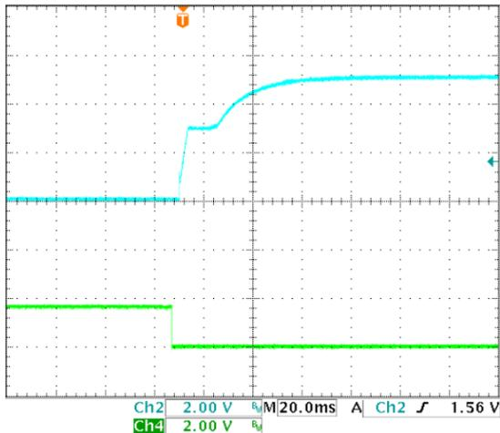
**Figure 4:** Turn-on transient at zero load current (20ms/div).  $V_{in}=48V$ . Top Trace:  $V_{out}$ ; 2V/div; Bottom Trace: ON/OFF input: 2V/div.
