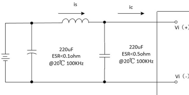
**Figure 10:** Test set-up diagram showing measurement points for Input Terminal Ripple Current and Input Reflected Ripple Current.
