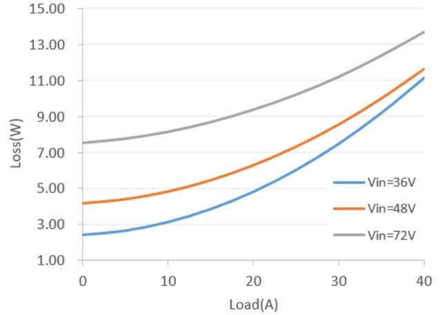
**Figure 2:** Power dissipation vs. load current for 36V, 48V, 53V and 72V input voltage at 25°C.
