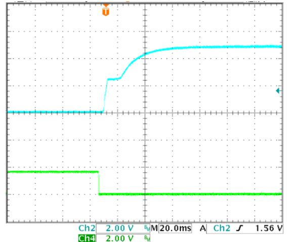
**Figure 5:** Turn-on transient at full load current (20ms/div).  $V_{in}=48V$ . Top Trace:  $V_{out}$ ; 2V/div; Bottom Trace: ON/OFF input: 2V/div.
