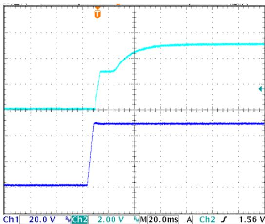
**Figure 6:** Turn-on transient at zero load current (20 ms/div). Top Trace:  $V_{out}$ ; 2V/div; Bottom Trace: input voltage: 20V/div
