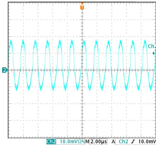
**Figure 14:** Output voltage ripple at nominal input voltage and max load current (10 mV/div, 2us/div)
