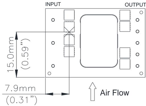
**Figure 18:** \* Hot spot 1's temperature measured point.
