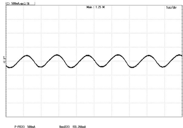
**Figure 11:** Input Terminal Ripple Current,  $i_c$ , at max output current and nominal input voltage with 12 $\mu H$  source impedance and 220 $\mu F$  electrolytic capacitor (500 mA/div, 1  $\mu s$ /div).
