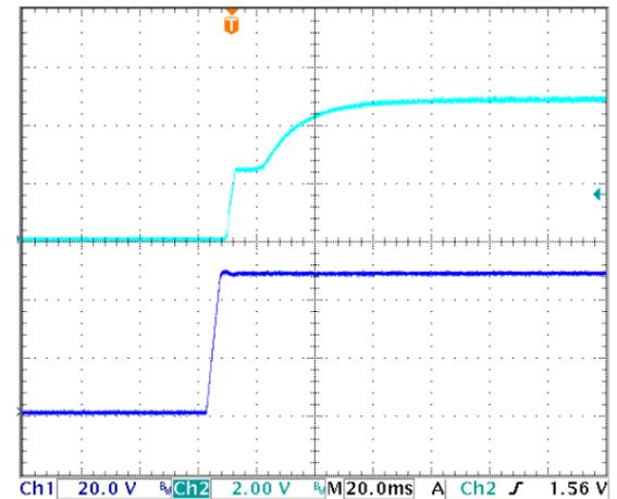
**Figure 7:** Turn-on transient at full load current (20 ms/div). Top Trace:  $V_{out}$ ; 2V/div; Bottom Trace: input voltage: 20V/div.
