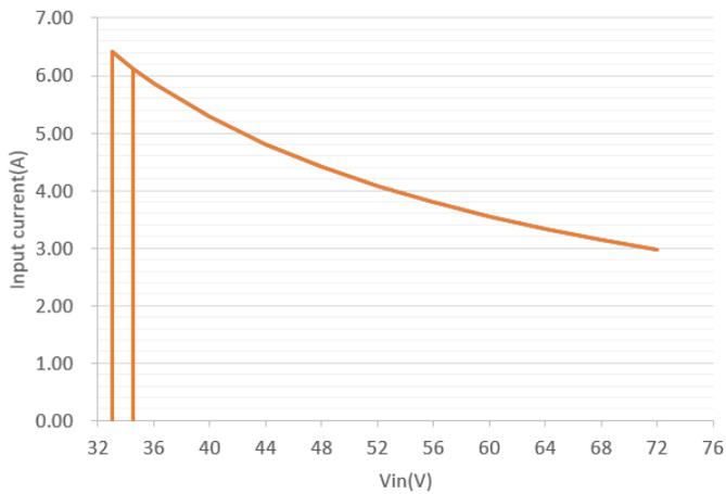
**Figure 3:** Full load input characteristics at room temperature.
