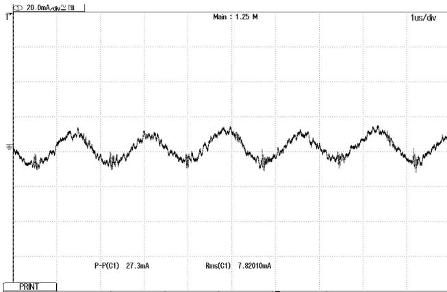
**Figure 12:** Input reflected ripple current,  $i_s$ , through a 12 $\mu$ H source inductor at nominal input voltage and max load current (20mA/div  $\cdot$  1us/div).
